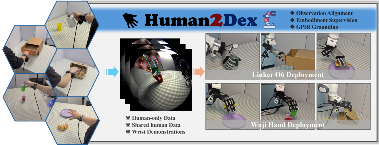
Fig. 1. Human2Dex overview. A wrist-mounted camera records natural bare-hand demonstrations. The shared wrist-centric observation and 21-point hand interface are converted offline into separate executable training sets for the Linker O6 and Wuji hands. Visual adaptation and GPIR provide shared interface semantics, whereas retargeting, action labels, normalization, and diffusion policies remain hand-task specific.
